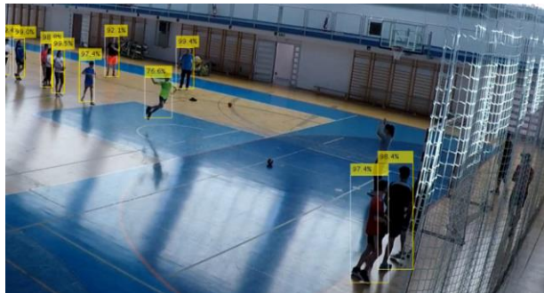
Figure 3. Bounding boxes with confidence values as results of Mask R-CNN person detection
