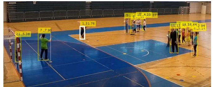
Fig. 5. Detected players (yellow box) and detected active player (white box). IDs and activity measures are shown above the boxes.
