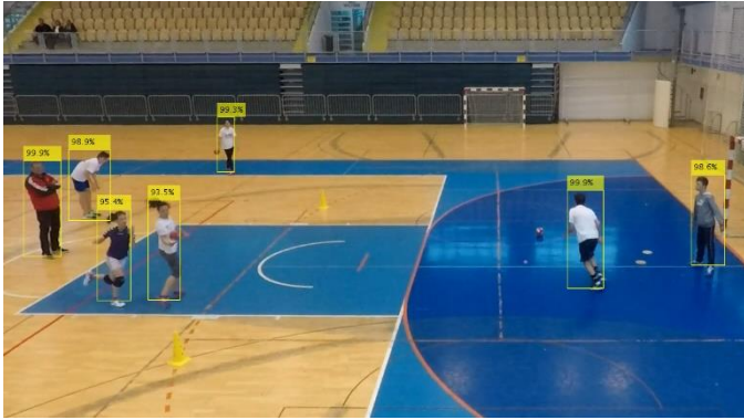
Fig. 3. Results of Mask R-CNN person detection
