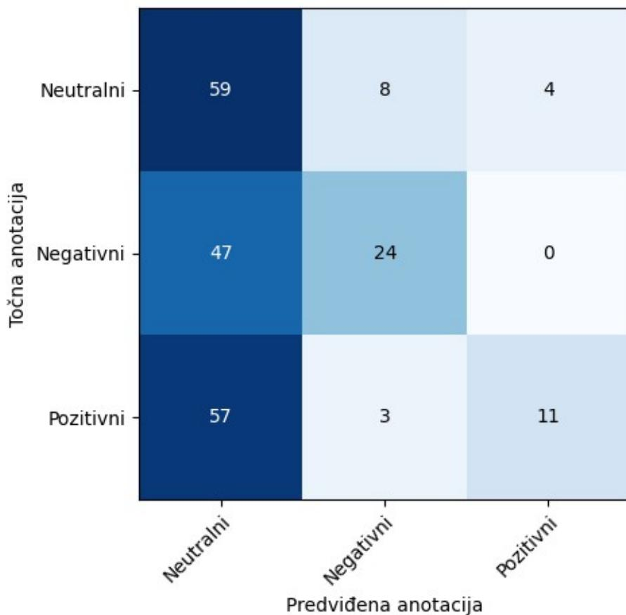
Slika 16: Matrica zabune - Support Vector Machine (balansirane klase)
