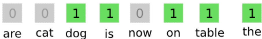
Slika 64. Pristup bag of words, preuzeto sa: https://miro.medium.com/max/451/1*eUedufA17_sI_QWSEIstZg.png
