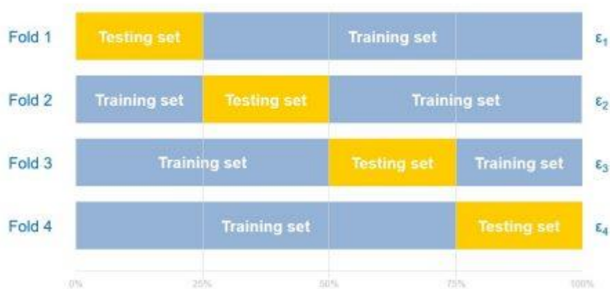
Slika 66. Unakrsna validacija, preuzeto sa: https://es.mathworks.com/discovery/cross-validation/jcr_content/mainParsys/image.adapt.480.medium.jpg/1611249630573.jpg
