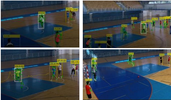
Fig. 9. Marking of the leading player (white thick bounding box); left is a correct detection and right is a wrong detection
