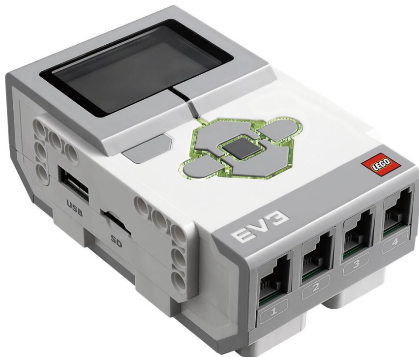
Slika 11: Lego EV3 Intelligent Brick
