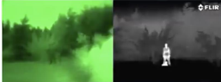
Fig. 1. Night vision vs. thermal imaging showing that tree camouflage cannot hide a person from a thermal camera 1 .
