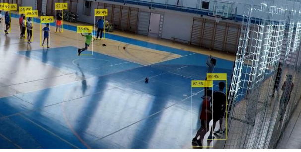
Fig. 2. Bounding boxes with confidence values as results of Mask R-CNN person detection
