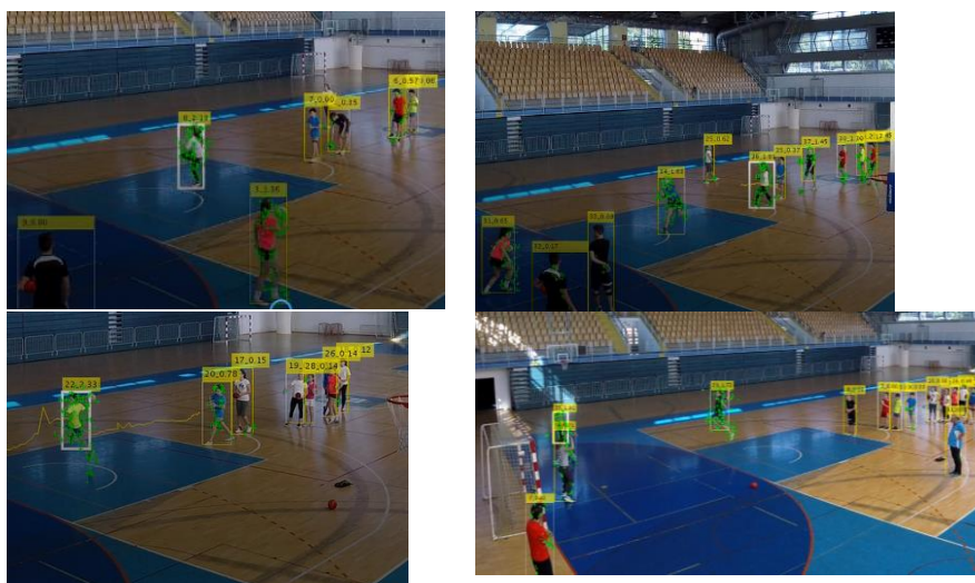
Figure 9. Marking of the leading player (white thick bounding box); left is a correct detection and right is a wrong detection
