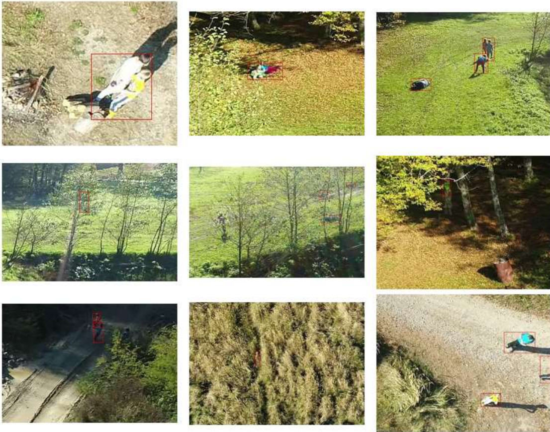
Figure 12. Miss detections of the YOLOv4 (SARD) model (cropped images to make it easier to notice the persons in the image): two people are standing very close to each other or overlapping (first row); darker parts of vegetation detected as a person (second row); shadows detected as persons (third row).
