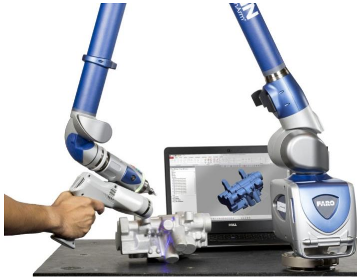
Slika 23: Sustav sa rukom i sondom (Izvor: https://www.indiamart.com/proddetail/faro-llp-3d-scanning-service-20657902348.html )
