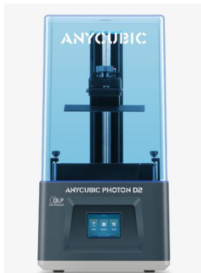
Slika 10: DLP 3D printer (Izvor: https://store.anycubic.com/products/photon-d2-dlp-3d-printer )
