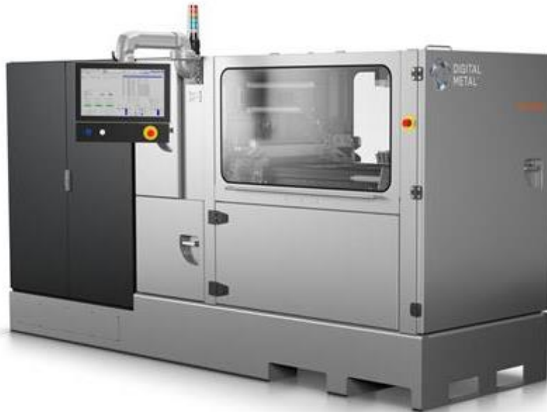
Slika 13: Slika Binder Jetting 3D printera (Izvor: https://amfg.ai/2018/04/27/top-5-binder-jetting-machines/ )
