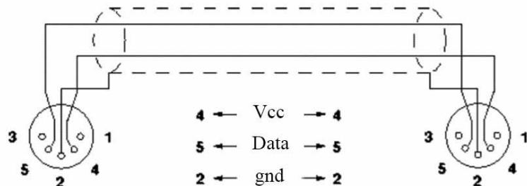
Slika 21 - MIDI 5 PIN DIN pinout shema
